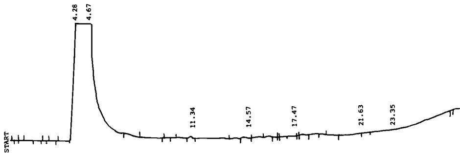
FIG. 1—Kapak/Scotchpak polyester pouch heated 4 h in metal can (convection oven, attenuation 32 \times 100 ).
